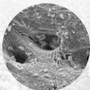
SEM image at 5000x magnification showing the microporous structure of CeraOss®.
